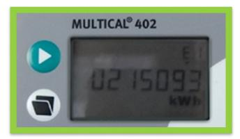
Example of a heat meter: normally located in an airing cupboard inside your property. This will display your joint heating and hot water usage in kWh.
